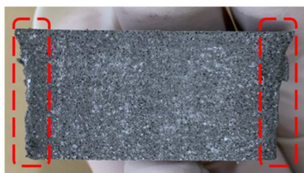
Figure 4. NENA enrichment in the interfacial propellant area.
