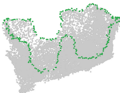
Figure 5. Example of hole boundary point detection result: the green points are the hole boundary points.
