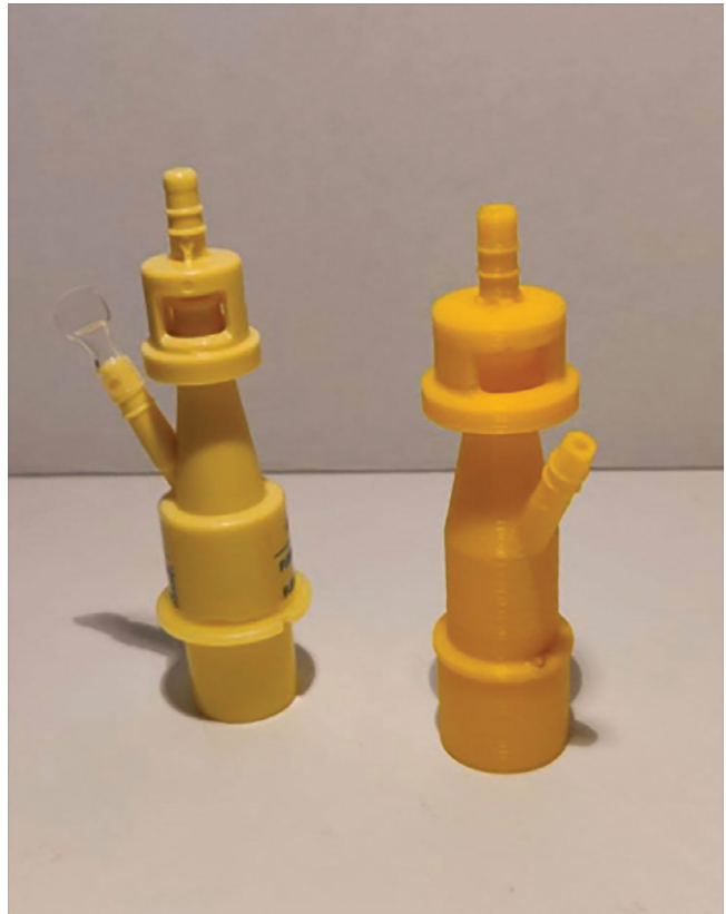
FIGURE 5 The original valve (on the left) and its 3D printed twin [Colour figure can be viewed at wileyonlinelibrary.com ]
