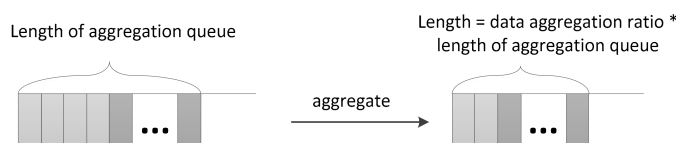
Figure 2. Length of the aggregation queue is reduced by aggregation.
