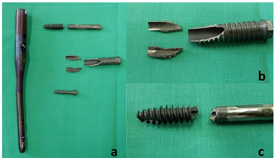
FIGURE 6: Broken implant (a), broken sleeve detail (b), and broken hip screw detail (c).
