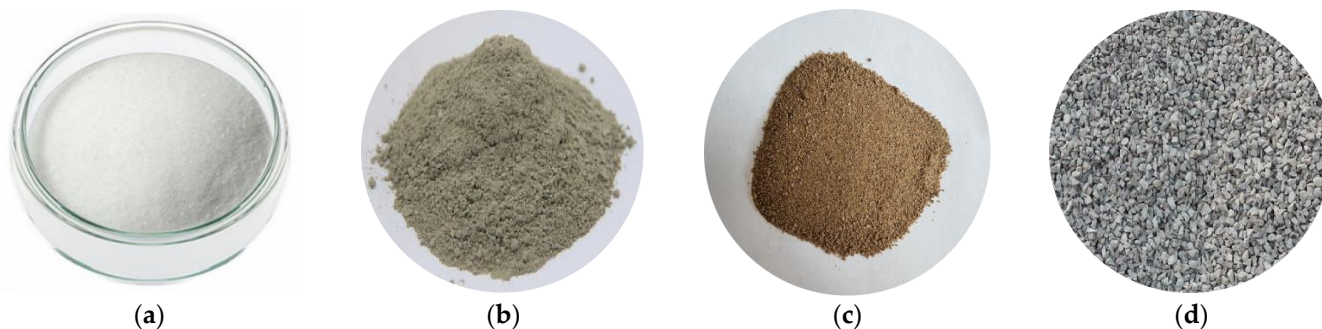
Figure 1. Test materials: (a) SAP; (b) cement; (c) fine aggregate; (d) coarse aggregate.
