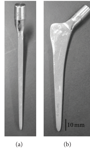
FIGURE 1: Duetto SI stem with a thin cross-sectional shape. (a) Medial side. (b) Arterial side. The stem surface was processed to produce 6-micron roughness in order to induce bone ongrowth.
