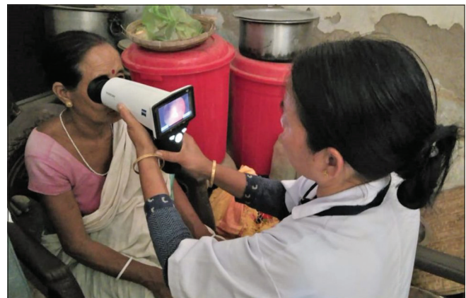
Figure 2: A field worker capturing a retinal image from a participant in the SMART-India study using a hand-held smartphone-based nonmydriatic retinal cameras (Zeiss Visuscout 100™)
