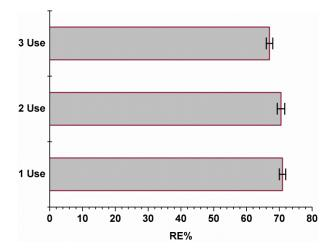
**Figure 3.** Bisphenol A removal efficiency, RE%, during regeneration and reuse of FF. Experimental conditions: fiber loading = 1 g; water volume = 50 mL;  $C_0 = 15$  mg/L; pH = 5; contact time = 60 min.
