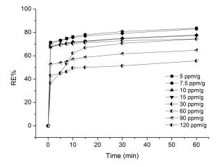
**Figure 5.** Process efficiency (%) in terms of BPA removal at various  $C_0/W$  (i.e., initial BPA concentration/fiber mass) ratios. Experimental conditions: water volume = 50 mL; pH = 5. The errors in the calculated removal efficiency are in the range from 0.11 to 1.17%.
