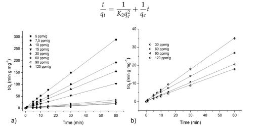
**Figure 6.** (a) Fitting of the experimental data by the pseudo-second order kinetics model. Experimental conditions: water volume = 50 mL; pH = 5. (b) Magnification of the data from 30 ppm/g to 120 ppm/g for a better visibility of the fitting. The errors in the  $t/q_t$  evaluations are in the range from 0.09 to 0.72%.
