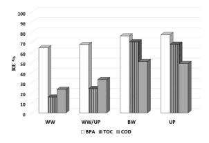
**Figure 4.** Removal efficiency, RE%, in various water matrices. Experimental conditions: fiber loading = 1 g; water volume = 50 mL;  $C_0$  = 15 mg/L; pH = 5; contact time = 60 min. The errors in the calculated removal efficiency are 1% for BPA, 2% for TOC and 4% for COD.
