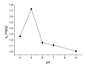
**Figure 2.** BPA equilibrium adsorption capacity  $q_e$  as a function of pH. Experimental conditions: fiber loading = 1 g; water volume = 100 mL;  $C_0$  = 30 mg/L; water matrix = UP.
