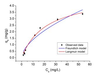
**Figure 7.** Bisphenol A adsorption isotherm at 20 °C onto biobased FF (black symbols) and fitting with the Langmuir (red line) and Freundlich (blue line) models.
