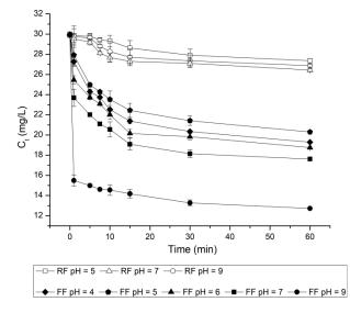
**Figure 1.** Effect of pH on the removal of Bisphenol A (BPA) by raw (RF) and functionalized (FF) fiber. Experimental conditions: fiber loading = 1 g; water volume = 100 mL;  $C_0 = 30 \text{ mg/L}$ ; water matrix = UP.
