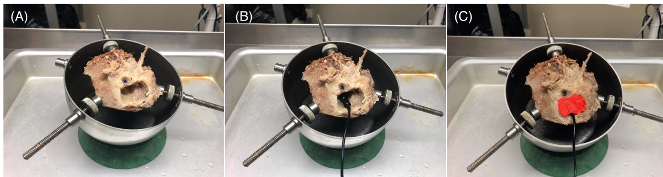
FIGURE 1 Temporal bone set up. A, Cadaveric temporal bone with mastoidectomy. B, Microphone placed into the retro-tympanic space in the mesotympanum. C, Modeling clay filling the mastoid cavity to form a neo-mastoid cortex
