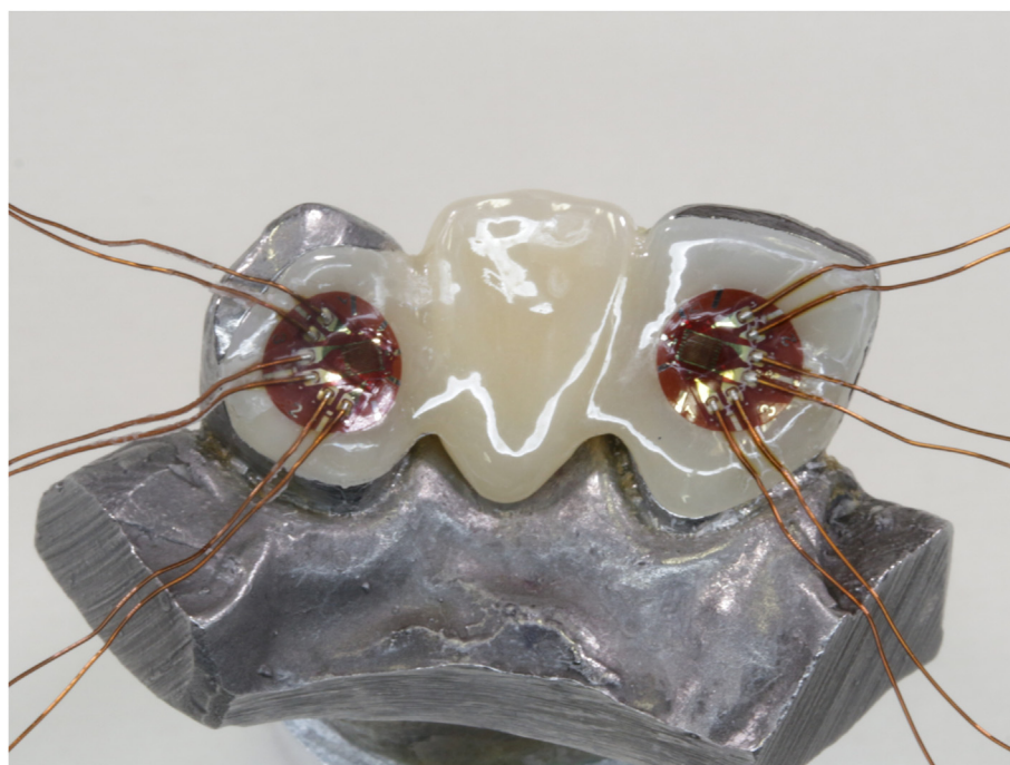
Figure 2 Strain gauges on each retainer.
