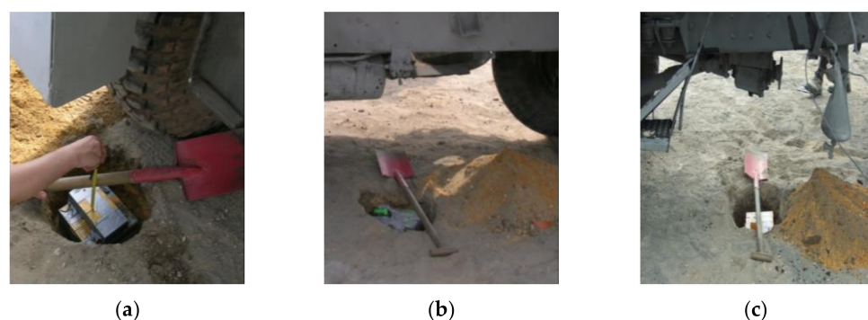
Figure 4. The load of TNT and its distribution during the first tests: (a) 10 kg of TNT under the wheel, (b) 10 kg of TN under the center of the hull, (c) and 10 kg of TNT under the reducer.
