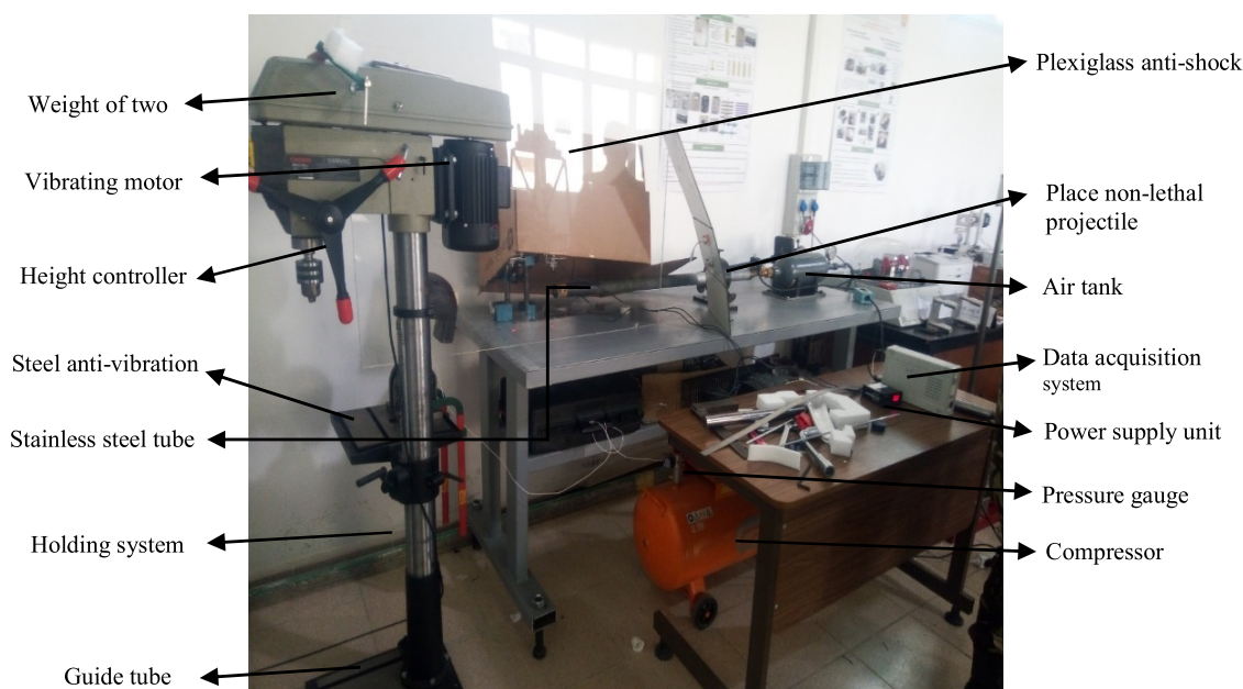
Figure 2. Overall sight of the pneumatic launcher.
