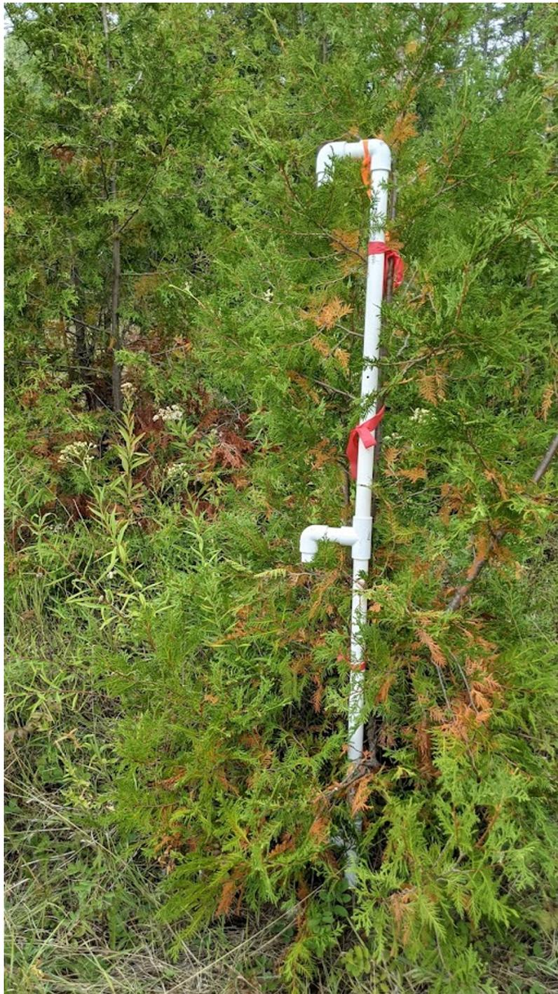
**Figure 1** Image of a PVC pole containing iButtons at 0.05 m, 0.75 m, and 1.5 m deployed in the field.
