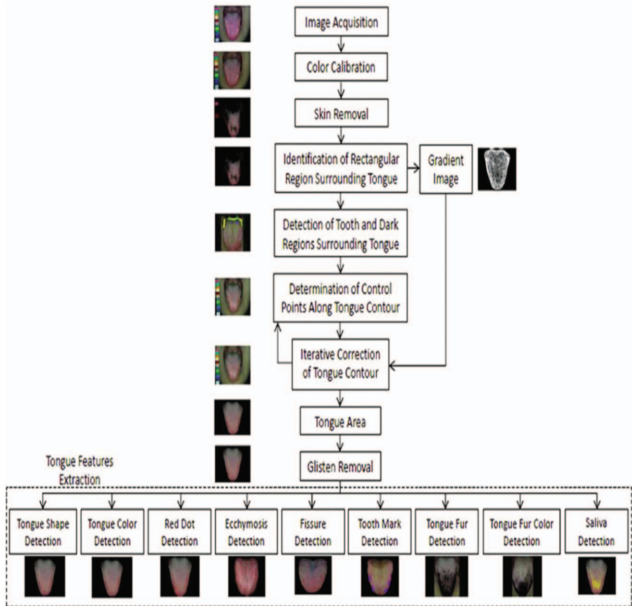
Figure 2. The processing steps of ATDS analysis.
