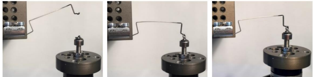
Figure 5. The three relevant positions of the cantilever during the measurements showed by the example of a 6 mm high utility arch. Left: neutral. Middle: activated. Right: 3 mm deactivated.
