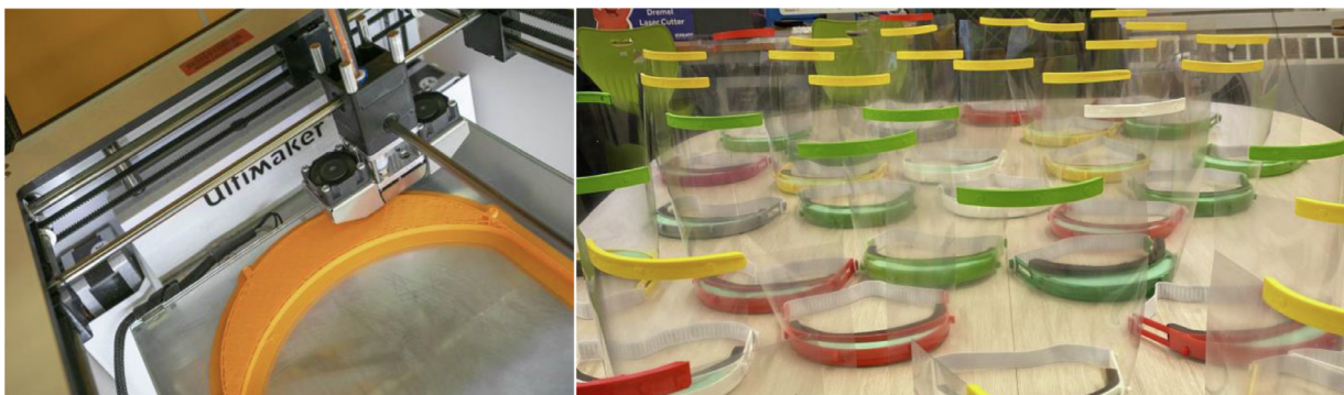
Fig. 9. Face shields printed through Stony Brook University iCreate for healthcare workers at Stony Brook Medical Center.
