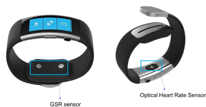
FIGURE 2. The Microsoft band and its sensors for GSR, heart rate, and skin temperature.
