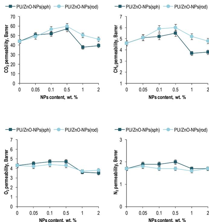
**Figure 6.** The permeability coefficients for the polymeric membranes based on the PU/ZnO-NPs.
