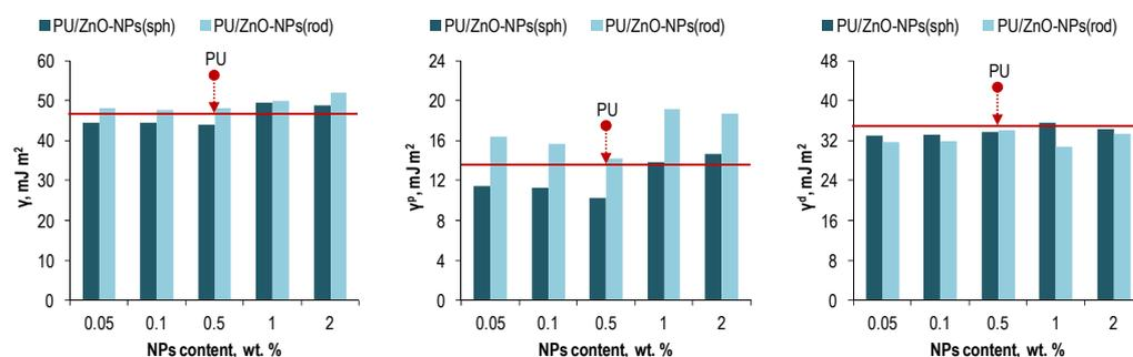
**Figure 5.** The specific surface free energy (overall (left), polar (center), and dispersive (right)).
