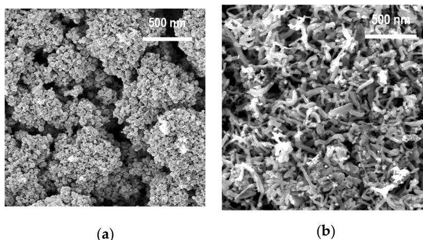
**Figure 2.** The SEM images of the spherical (a) and rod-shaped (b) ZnO-NPs obtained by the PECVD method.
