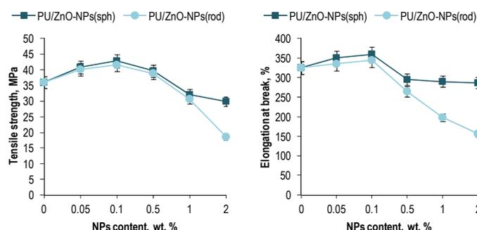
**Figure 8.** The mechanical properties of the polymeric membranes based on the PU/ZnO-NPs.
