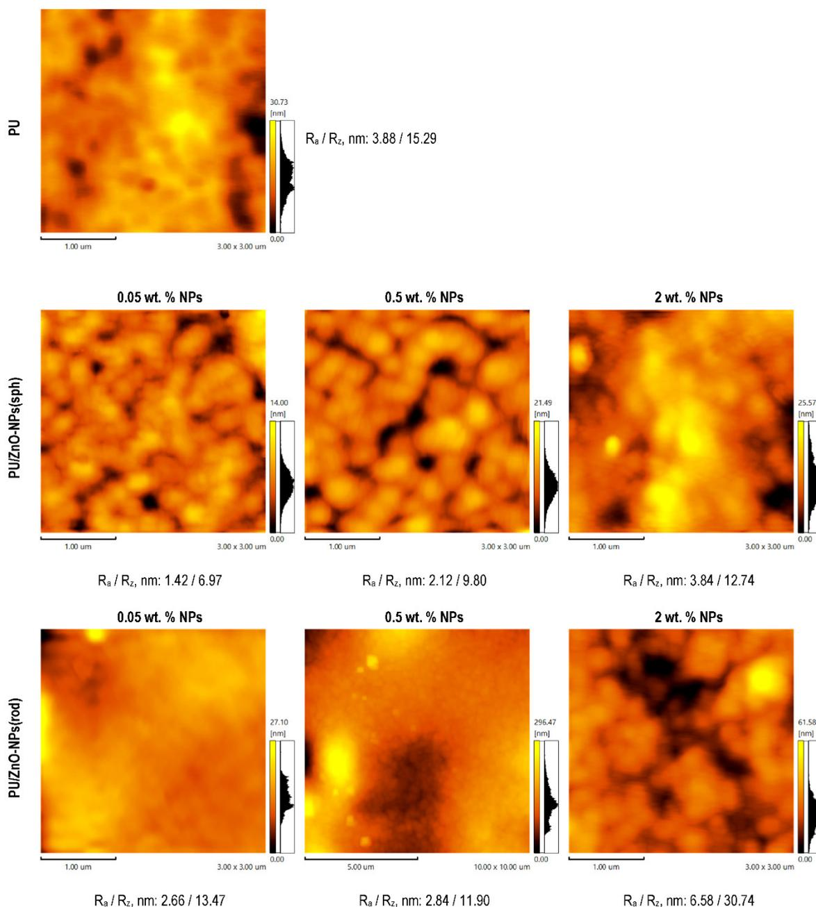
**Figure 4.** The AFM data of the membranes based on the various PU solutions with ZnO-NPs.
