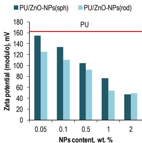
**Figure 3.** The zeta potential of the polymer solutions based on PU/ZnO-NPs in THF.
