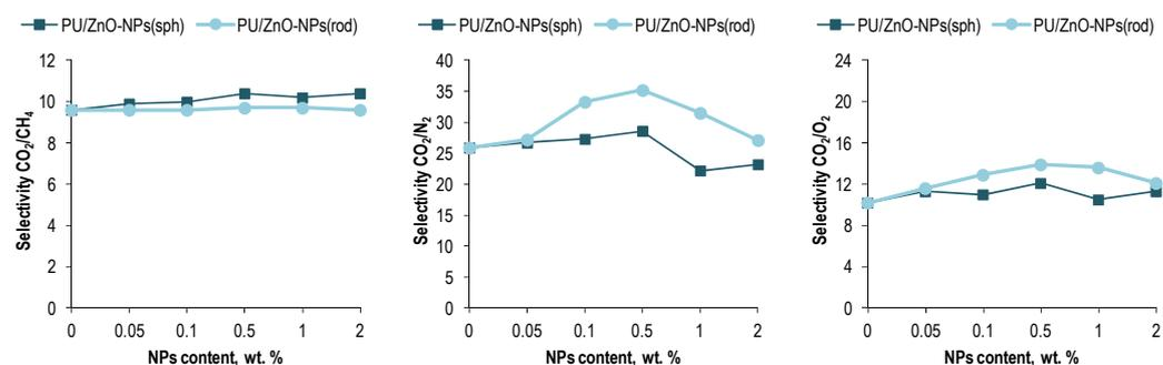
**Figure 7.** The selectivity of the polymeric membranes based on the PU/ZnO-NPs.
