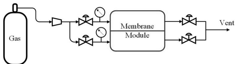
**Figure 1.** The scheme of the experimental setup for gas separation testing.
