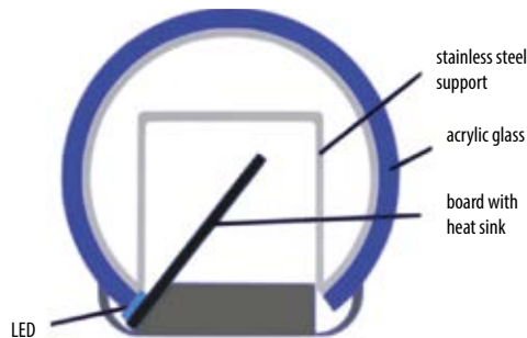
Fig. 4 Schematic cross-sectional drawing of the antimicrobial LED handrail.
