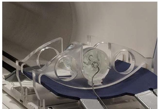
**FIG. 2.** ViewRay QA cylindrical water phantom setup used to investigate directional dependence using ionization chamber and metal-oxide-semiconductor field-effect transistors (MOSFET).
