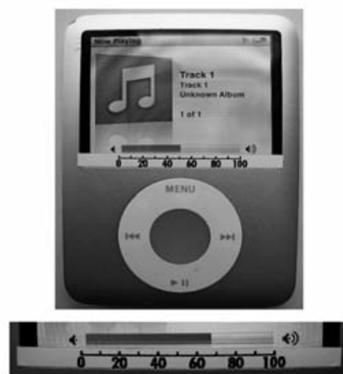
Figure 1. Image of the scale indicating percentage values in increments of 10 from 0 to 100 that was fixed to the display screen of the iPod. The value represents the volume bar setting, not the actual sound pressure level output level.
