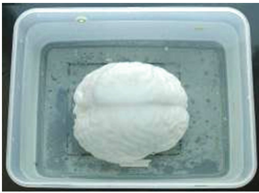
Fig. 4 The brain phantom was fixed in one Plexiglas box with five fiducial landmarks. It has a similar shape to the human brain and similar linear elastic parameters of Young's elasticity modulus and Poisson's ratio as the human brain to ensure that the phantom has the similar elastic behavior as the brain
