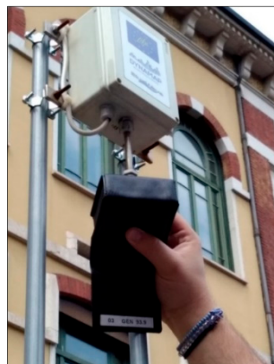
Figure 10. Operation of calibration on DYNAMAP sensor.
