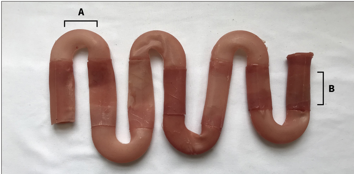
Fig. 2. Small intestine model. U-shaped connectors (A) are used to connect straight joints (B).
