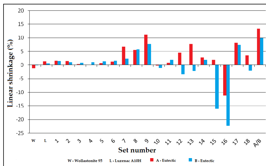
Figure 9. Comparison of the linear shrinkage of the A/B eutectic–wollastonite–talc.
