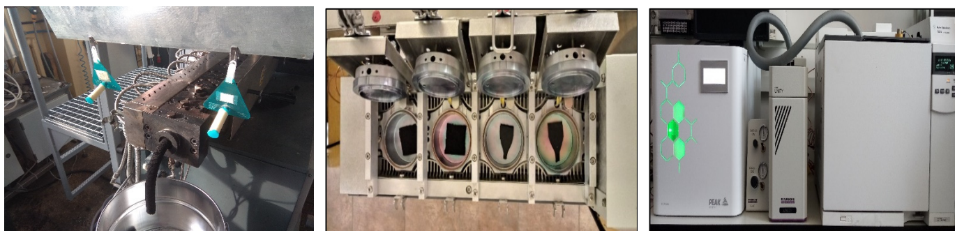
Figure 5. The appearance of the apparatus for determining the TVOCs parameter; from left: Radiello ® passive 5 sampling system; Micro-Chamber/Thermal Extractor TM ; gas chromatograph.
