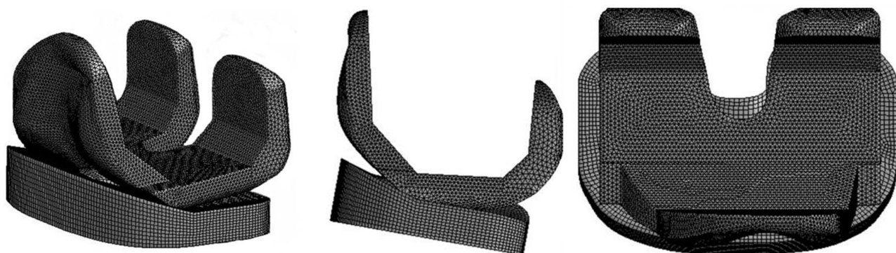
Figure 1 Three-dimensional models of the femoral component, sensor, and PE insert.
