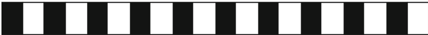
Fig. 1. Two-periodic pattern in the ECA composed by 20 cells. The binary expression for all these rules has the form: xx0xx1xx , where x can be either 0 or 1. That is, the pattern consisting of a repetition of black and white remains the same when the transition rule leaves the configurations 3 and 6 unaltered: (010) \rightarrow (010) and (101) \rightarrow (101) .
