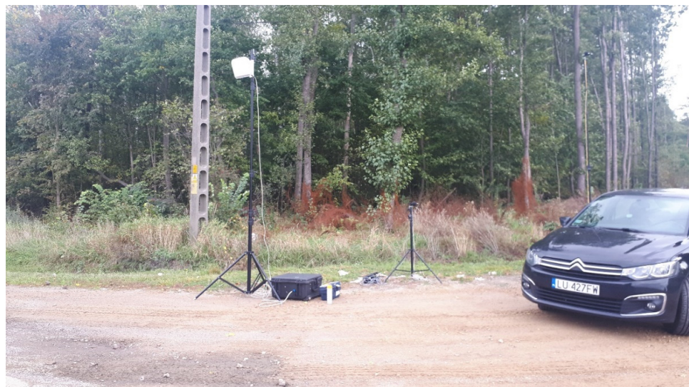
Figure 2. View of the test stand used for the SPB testing method in in situ conditions.
