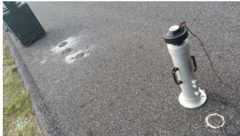
Figure 4. View of the location of the impedance tube during testing in relation to the surface sample collection site.
