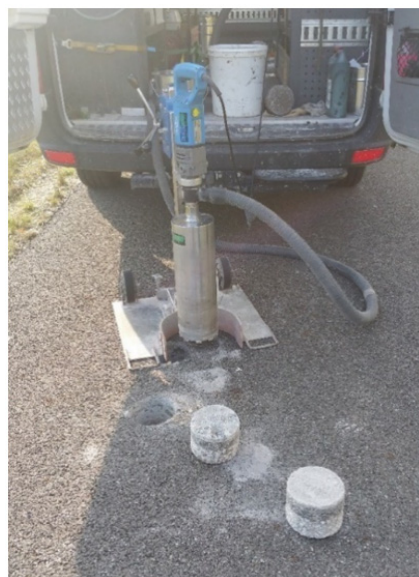
Figure 3. View of samples taken at the site of measurements in the research section in Bolimów.
