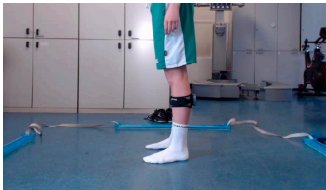
Figure 1. Subject equipped with the inertial sensor on the black stripe and placed within the area defined by the optoelectronic bars.
