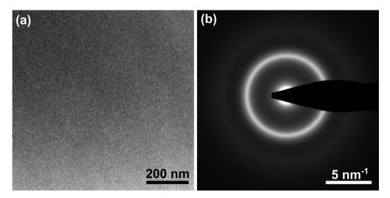
Figure 2. TEM images of  $Cu_{46.5}Zr_{46.5}Al_5Ag_2$  BMG. Bright field-image (a) and the corresponding selected area diffraction pattern (b) taken from a large area of the  $Cu_{46.5}Zr_{46.5}Al_5Ag_2$  BMG sample reveal a homogeneous amorphous structure without the presence of nanocrystals.
