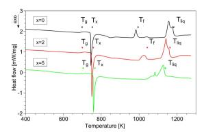
Figure 5. Differential calorimetry curves (heating rate 20 K/min) of the various CuZrAl(Ag) BMG (for clarity the curves are shifted vertically). The glass transition temperature  $T_g$ , the crystallization temperature  $T_x$ , the final B2 transformation temperature  $T_f$  and the liquidus temperature  $T_{liq}$  are indicated. The decreasing temperature interval  $T_{liq}$ - $T_f$  with increasing Ag content indicates destabilization of the B2 phase.
