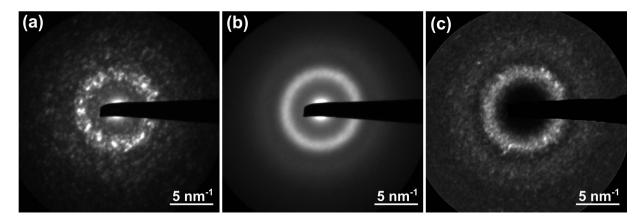
**Figure 1. Example of the nanodiffraction FEM. (a)** Representative nanodiffraction pattern extracted from the dataset acquired on the Ag-free  $Cu_{47.5}Zr_{47.5}Al_5$  alloy with a beam size of 1.2 nm. (b) Average of all nanodiffraction patterns in the dataset. (c) Normalized intensity variance calculated for each pixel across the entire dataset.
