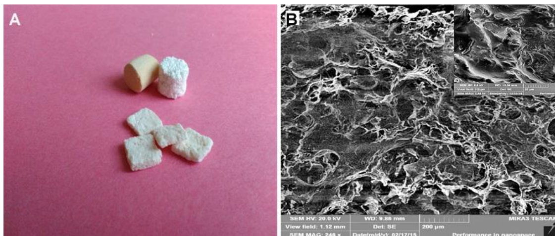
Figure 1. PHB/CHIT biomaterial. (A)—Macroscopic design of the used scaffold for the filling of the osteochondral defect; (B)—Microstructure of PHB/CHIT scaffold with pores (SEM), scale bar: 200 \mu\text{m} .
