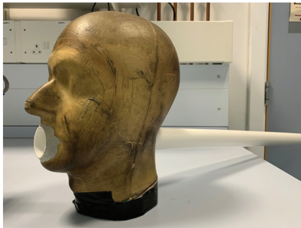
Figure 4. Cough simulator cough delivery point attached to the 'wearer' manikin head.
