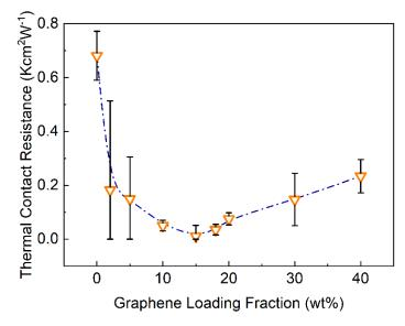
**Figure 5.** Thermal contact resistance,  $R_C$ , of TIMs as a function of the graphene loading,  $\xi$ . Note the non-monotonic dependence of  $R_C$  on graphene loading. The bars show the standard error of the linear fittings used for data extraction.
