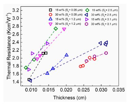
**Figure 6.** Thermal resistance,  $R_{tot}$ , of the graphene TIM dispersed between two copper plates as a function of the bond line thickness, BLT. The results are presented for two different graphene loadings,  $\xi$ , and four different values of roughness,  $S_q$ . In each measurement, the two copper plates used had the same roughness. The dashed lines show the linear regression fittings to the experimental data.
