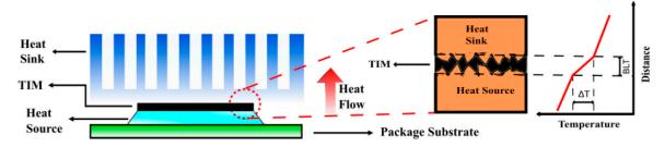
**Figure 1.** Schematic representation of a packaged device illustrating the role of TIMs. TIM is applied between the adjoining heat source and the heat sink surfaces in order to fill the air gaps and facilitate the heat transfer.
