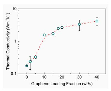
**Figure 4.** Thermal conductivity,  $K_{TIM}$ , of TIMs as a function of graphene loading fraction,  $\xi$ . Adding graphene fillers to the noncuring oil base increases the "bulk" thermal conductivity of graphene TIMs. The bars show the standard error of the linear regression slope.
