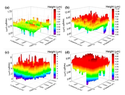
**Figure 2.** Roughness characteristics of the copper plates determined by an optical profilometer. The plates have the following root mean square (RMS) roughness: (a)  $S_q = 0.05 \, \mu \text{m}$ , (b)  $S_q = 1.2 \, \mu \text{m}$ , (c)  $S_q = 2.5 \, \mu \text{m}$ , and (d)  $S_q = 3.1 \, \mu \text{m}$ .
