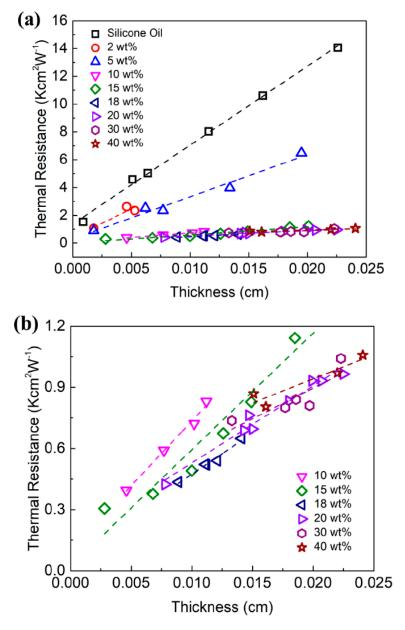
**Figure 3.** Total thermal resistance,  $R_{tot}$ , of graphene TIMs as a function of the bond line thickness, BLT. The dashed lines show the linear regression to the experimental data used to extract the thermal conductivity,  $K_{TIM}$ , and thermal contact resistance,  $R_C$ . (a) Thermal resistance vs. BLT for all tested loading fractions of graphene and pure silicone oil base. (b) Thermal resistance vs. BLT for loading fractions of  $\xi = 10$  wt% and above are shown for clarity.
