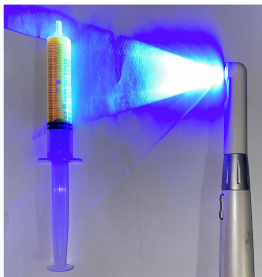
Figure 3. The light source. A commercialized curing light was used as a light source for blue light fluorescence.
