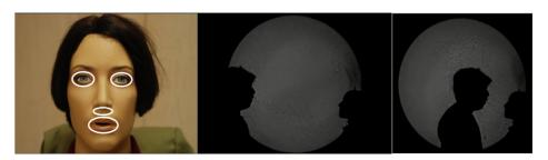
**Figure 2. Singapore experimental set-up, showing:** Swabbing sites for the manikins' face (A) for influenza testing. Shadowgraph images of far-(B) and near- cough (C) distances (see accompanying online Video S1 for further details of these shadowgraph images). doi:10.1371/journal.pone.0107338.g002
