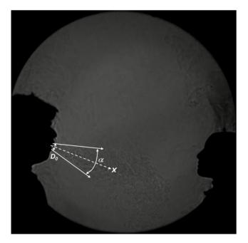
Figure 3. Example of cough shadowgraph image showing the dispersal of the exhaled puff. Parameters that affect the dispersal of this exhaled airflow include the mouth-opening diameter ( $D_0$ ), propagation distance (x), and spreading angle ( $\alpha$ ) (see accompanying online Video S1 for further details of these shadowgraph images). doi:10.1371/journal.pone.0107338.g003
