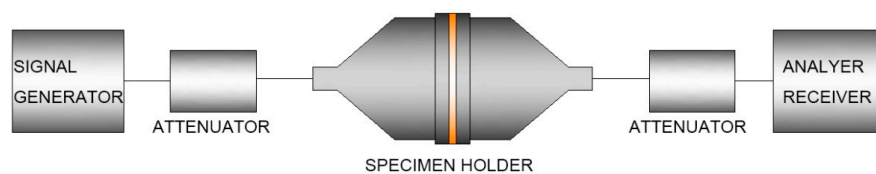
Figure 1. Schematic diagram of flange coaxial transmission line device for electromagnetic interference (EMI) shielding effectiveness (SE) test.
