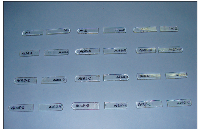
Figure 3: Fractured samples after testing
