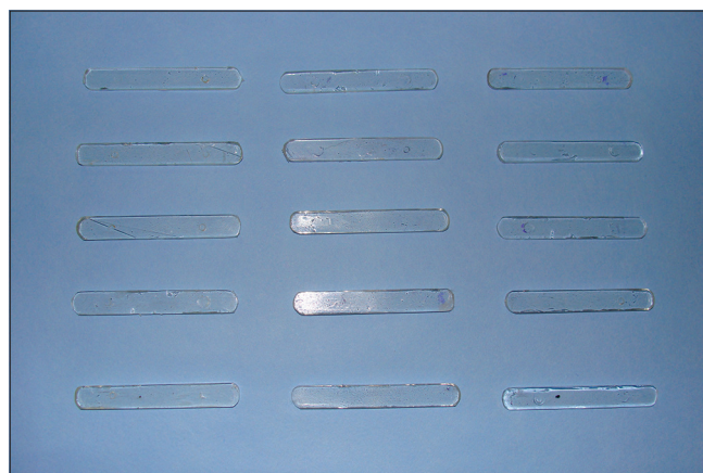
Figure 1: Finished and polished samples for flexural strength
