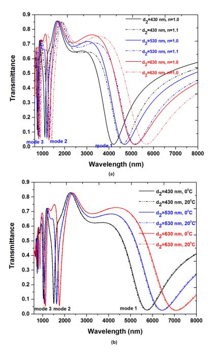
**Figure 7.** Transmittance spectra as a function of the (**a**) RI (n = 1.0 and 1.2) and (**b**) ambient temperature (T = 0 °C and 20 °C) for different d<sub>2</sub> (i.e., 430 nm, 530 nm and 630 nm) of the MIM waveguides. The other parameters are kept the same as used in Figure 2.
