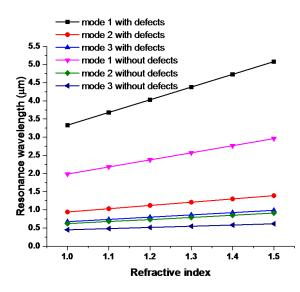
**Figure 3.** Resonant wavelengths versus the refractive index (RI) with and without silver nanorod defects in T-shape cavity.
