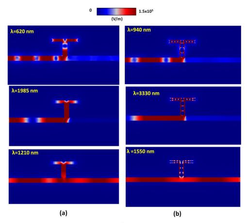
**Figure 4.** Electric field intensity ( $|E| = (E_x^2 + E_y^2)^{1/2}$ ) for the cases (**a**) without defects (at  $\lambda_{res} = 620$  nm, 1985 nm and 1210 nm) and (**b**) with defects (at  $\lambda_{res} = 940$  nm, 3330 nm and 1550 nm), respectively.
