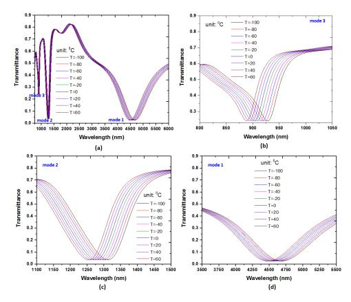
**Figure 5.** (a) Transmittance spectrum of the proposed MIM plasmonic waveguide with different ambient temperature in the wavelength range of 700–6000 nm. Transmittance spectrum of the proposed MIM plasmonic waveguide with different ambient temperature (b) in the wavelength range of 888–928 nm for mode 3, (c) in the wavelength range of 1254–1312 nm for mode 2, and (d) in the wavelength range of 4478–4688 nm for mode 1, respectively. The other parameters are set as the same as used in Figure 2.
