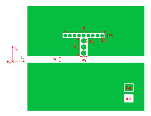
**Figure 1.** Schematic diagram of the proposed metal–insulator–metal (MIM) sensor structure coupled with several silver nanorod defects in a T-shape cavity.
