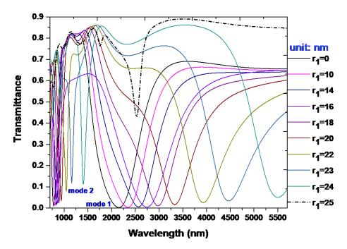
**Figure 6.** Transmittance spectra for different radius of the silver nanorods with  $r_1 = (0, 8, 10, 12, 14, 16, 18, 20, 22, 23, 24, 25)$  nm, respectively. The other parameters are set as the same as used in Figure 2.
