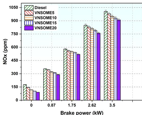
Figure 9.  $\text{NO}_x$  variation of the test fuels.
