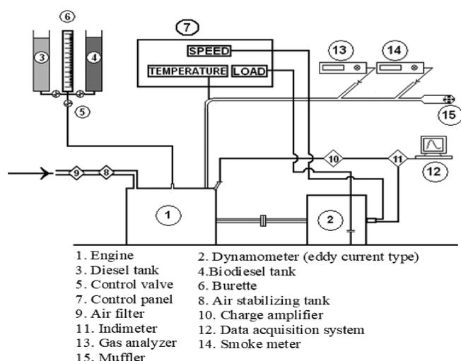
Figure 3. Schematic diagram of the test engine setup.
