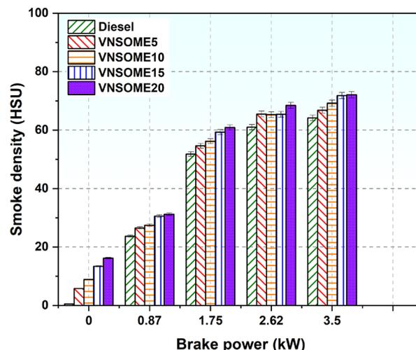
Figure 10. Smoke variation of the test fuels.
