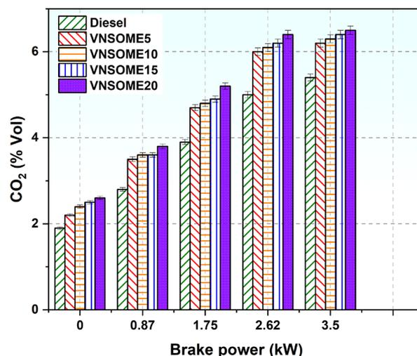
Figure 11.  $\text{CO}_2$  variation of the test fuels.
