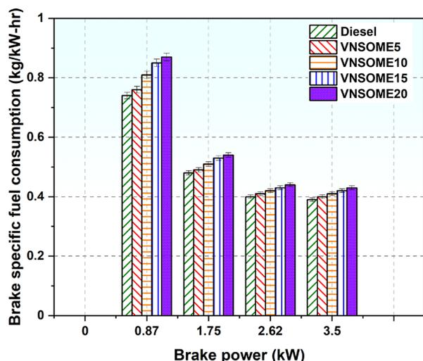
Figure 4. BSFC variation of the test fuels.
