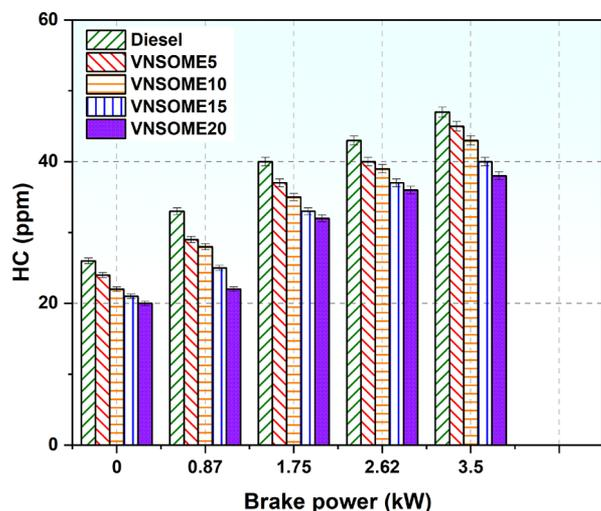
Figure 8. HC emission variation of the test fuels.
