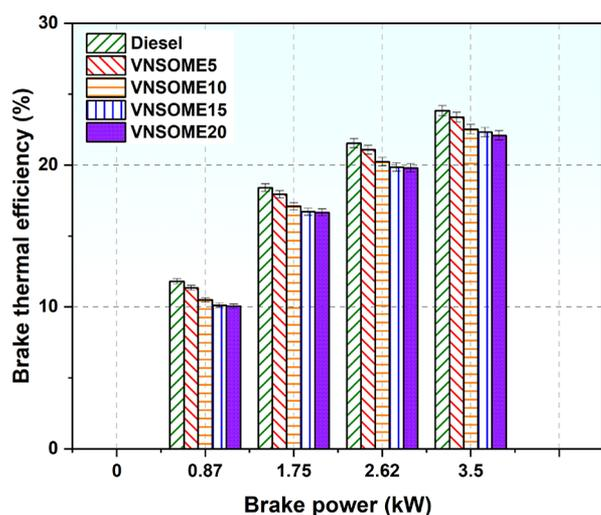
Figure 5. BTE variation of the test fuels.
