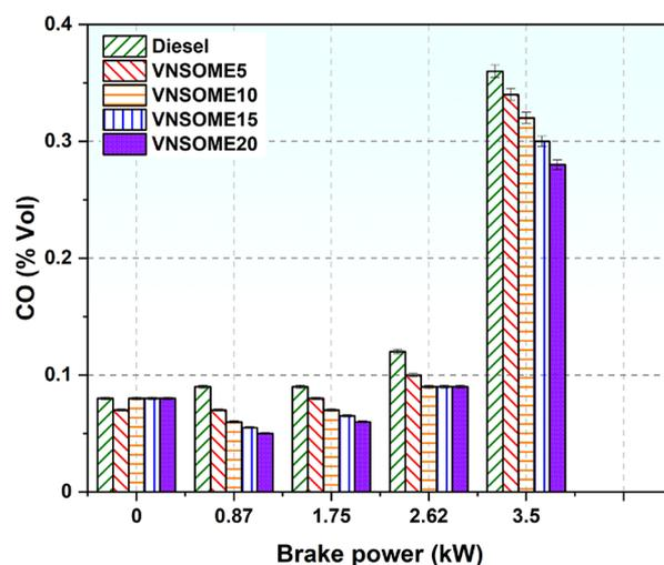
Figure 7. CO emission variation of the test fuels.
