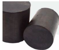
Figure 5. The ZN-1 viscoelastic material standard test piece.
