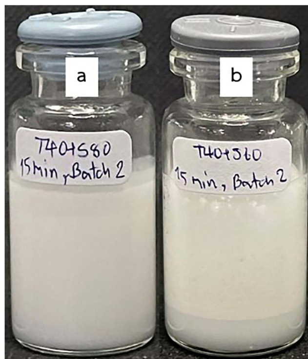
Figure 2 The physical appearance of emulsion after left 24-hr equilibrium: (a) Slightly creamy emulsions (b) Two-layer emulsions.
