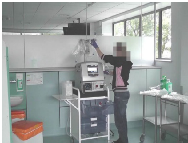
Figure 2 Test room set-up for Human Factors Testing of the Quanta SC+ home hemodialysis system [Color figure can be viewed at wileyonlinelibrary.com ]
