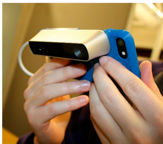
Figure 2. A user is holding an iPhone with the Structure Sensor.
