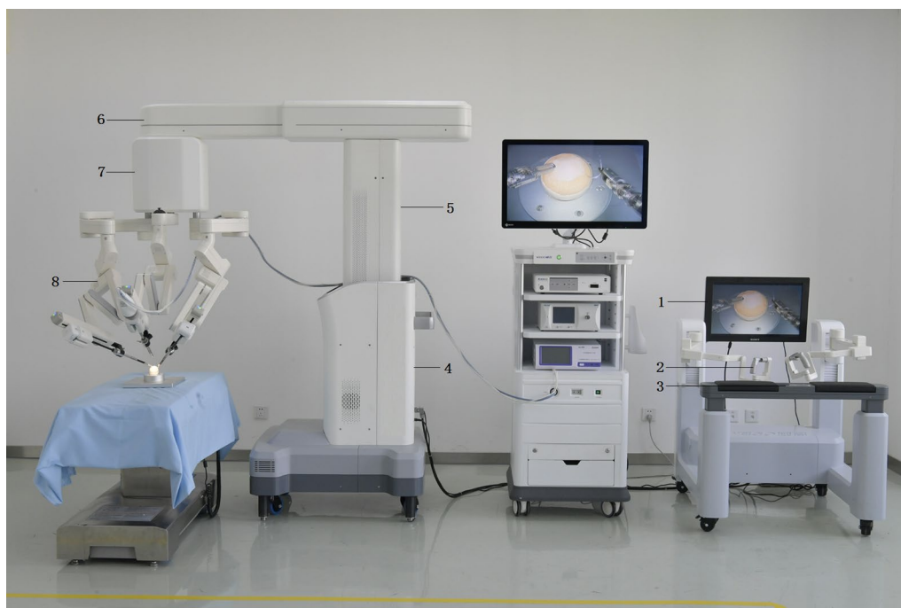
Fig. 1 The Micro Hand S surgical robotic system. Surgeon console (right): (1) image display device, (2) master arm, (3) control panel. 3D imaging system (middle). Slave surgical cart (left): (4) electrical control system, (5) lifting column, (6) suspension passive arm, (7) swivel head, (8) slave arm
