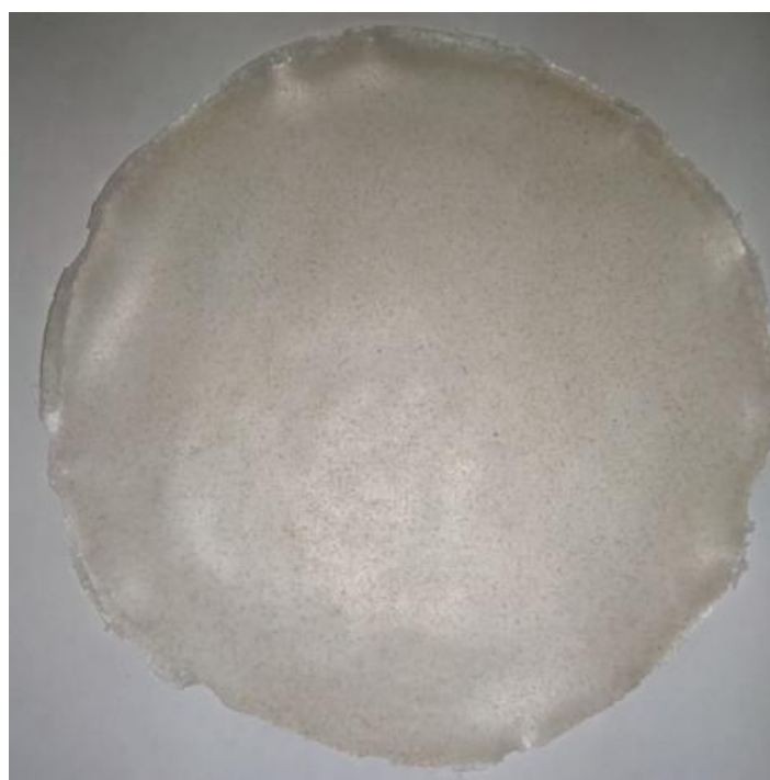
Figure 2. Corn starch biocomposite film reinforced with kenaf fibre.
