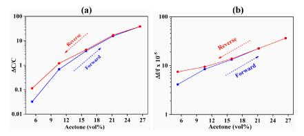
**Figure 6.** Hysteresis of (**a**) capacitive-based and (**b**) QCM-based sensors. The desorption cycle lagged behind the adsorption cycle by a maximum of approximately 3 vol % at 5.3 vol % of acetone.
