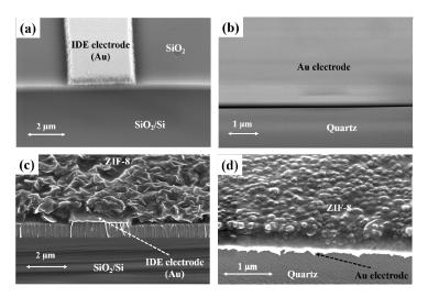
**Figure 3.** SEM micrographs before and after coating of the ZIF-8 film onto the sensing substrates obtained at a 45° tilt angle. (**a**) Uncoated interdigitated electrode (IDE) capacitive substrate. (**b**) Blank QCM substrate coated. (**c**) IDE capacitive substrate coated with ZIF-8 film. (**d**) QCM substrate coated with ZIF-8 film.
