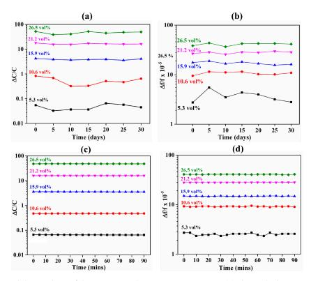
**Figure 7.** Stability analysis of the ZIF-8-coated sensors to acetone gas. (**a**) Shows the long-term stability of the capacitive sensor for 30 days. (**b**) Shows the long-term stability of the QCM-based sensor for 30 days. (**c**) Shows the short-term stability of the capacitive sensor. (**d**) Shows the short-term stability of the QCM-based sensor.
