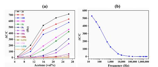
**Figure 11.** Effect of alternating current (AC) drive frequency on the sensitivity of the ZIF-8-coated IDE-based capacitive acetone sensor. (a) Sensitivity response of the sensor to acetone at various AC drive frequencies (20 Hz to 2 MHz). (b) AC drive frequency vs. sensitivity of the sensor at 15.9 vol % acetone.
