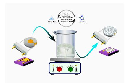
**Figure 1.** Schematic showing the mechanism used for growing zeolitic–imidazolate framework (ZIF-8) thin films on sensing substrates. The films were deposited by cyclic immersion in a 10-mL mixture of 25 mMol zinc nitrate hexahydrate (5 mL) and 50 mMol 2-Methylimidazole methanolic (5 mL) precursor solutions of [65].
