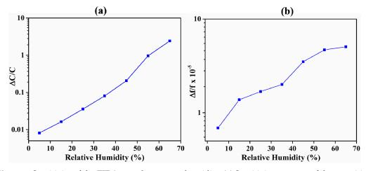
**Figure 8.** Sensitivity of the ZIF-8-coated sensors to humidity. (**a**) Sensitivity response of the capacitive sensor. (**b**) Sensitivity response of the QCM-based sensor.
