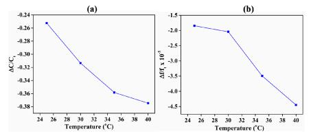
**Figure 9.** Sensitivity of the ZIF-8-coated sensors to changes in temperature. The acetone was fixed at 15.9 vol %. (a) Response of the capacitive sensor. (b) Response of the QCM sensor.
