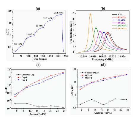
**Figure 5.** Response of the ZIF-8-coated and uncoated sensors to acetone gas. (**a**) This shows the typical response of the ZIF-8-coated capacitive sensors. (**b**) This shows the typical response of the ZIF-8-coated QCM-based sensors. (**c**) This shows the sensitivity of the two ZIF-8-coated (Cap-1 and Cap-2) and uncoated IDE capacitive sensors. (**d**) This shows the sensitivity of the ZIF-8 coated (QCM-1 and QCM-2) and uncoated QCM-based sensors.
