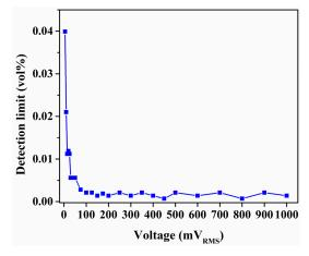
**Figure 10.** Tunability of the limit of detection by changing the drive voltage in the case of IDE-based capacitive acetone sensor.
