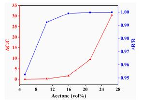
**Figure 12.** Comparison of changes in resistance vs. capacitance of ZIF-8 film coated onto IDE-substrate-based acetone sensors. The capacitance and resistance values were measured at 100 kHz.
