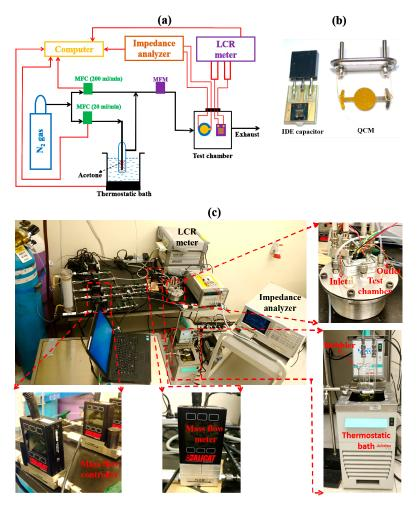
**Figure 2.** Experimental setup for gas sensing. (a) Schematic of the experimental setup used for characterizing and comparing the gas sensors. (b) Digital image of the capacitive and quartz crystal microbalance (QCM) substrates coated with ZIF-8 thins film. (c) Digital image of the experimental setup.
