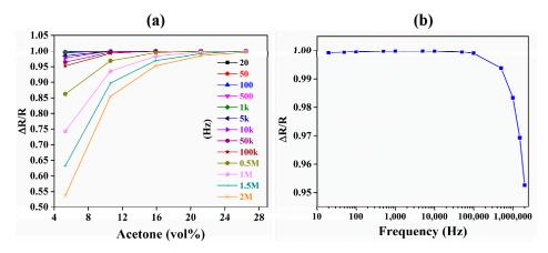
**Figure 13.** Changes in the device sensitivity vs. actuation frequency for resistive transduction. (a) This shows the change in device response at different actuation frequencies. (b) This shows the change in device sensitivity with increases in drive frequency at 15.9 vol % of acetone in N<sub>2</sub>.
