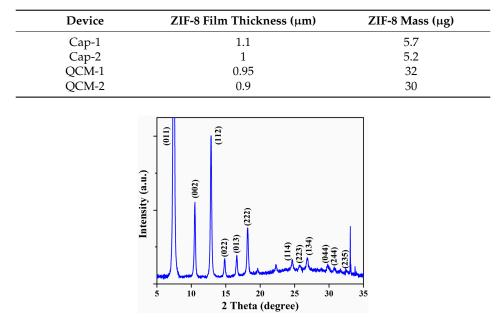
Figure 4. Shows the XRD pattern of a ZIF-8 thin film grown using the cycle method.
