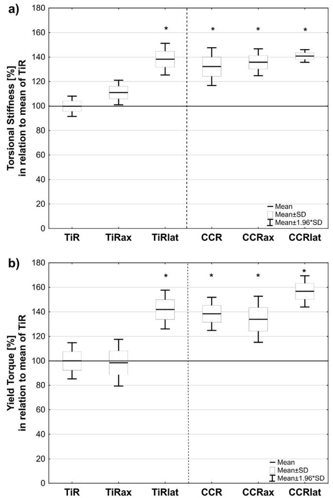
**Fig. 4.** Results of all tested configurations normalized to the results of TiR for static torsional loading according to ASTM F1717-21: a) torsional stiffness b) yield torque. \*Statistically significant difference compared with TiR.
