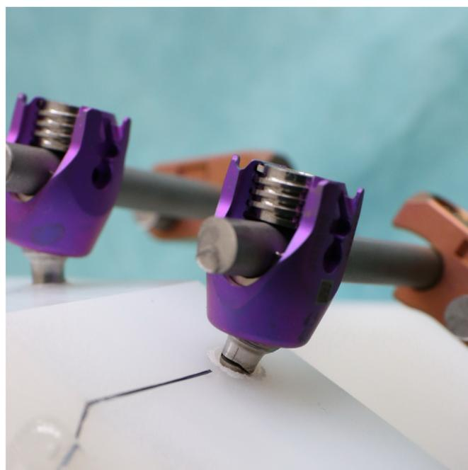
Fig. 7. Typical failure mode of a cobalt chromium rod construct: screw breakage.
