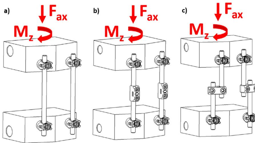
**Fig. 2.** Vertebrectomy constructs according to ASTM F1717-21 for the six different instrumentation types: a) standard configuration of pedicle screw rod construct (TiR, CCR), b) axial rod connector configuration (TiRax, CCRax) and c) lateral connector (TiRlat, CCRlat).
