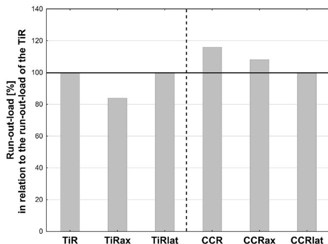
Fig. 5. Run-out-load levels for the different test groups in relation to the run out load level of TiR (run out load level of TiR is equal to 100%).
