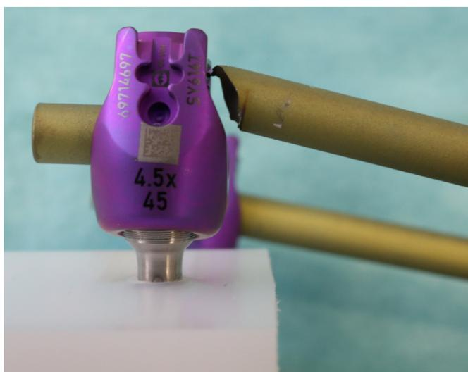
Fig. 6. Typical failure mode of a titanium rod construct: rod breakage.
