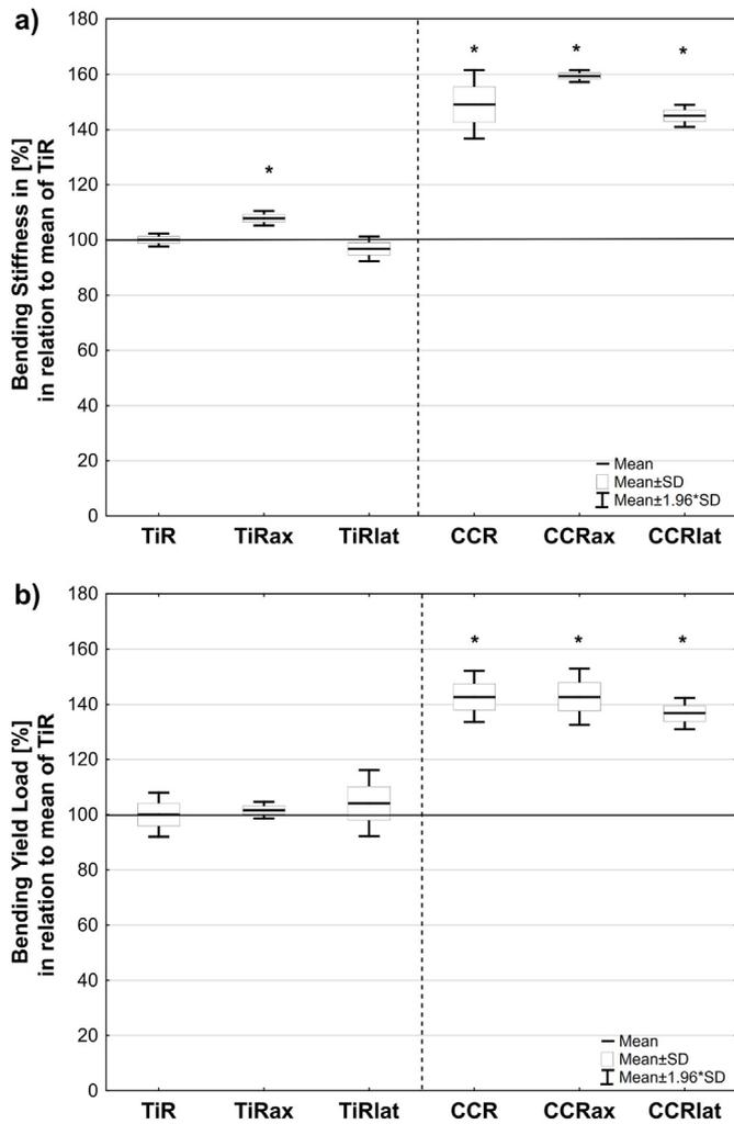
**Fig. 3.** Results of all tested configurations normalized to the results of TiR for static compression bending loading according to ASTM F1717-21: a) bending stiffness b) bending yield load. \*Statistically significant difference compared with TiR.
