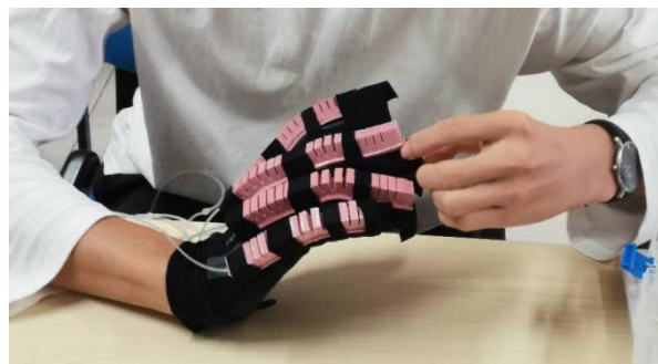
Figure 1. The design of the soft exoskeleton glove (SExoG).
