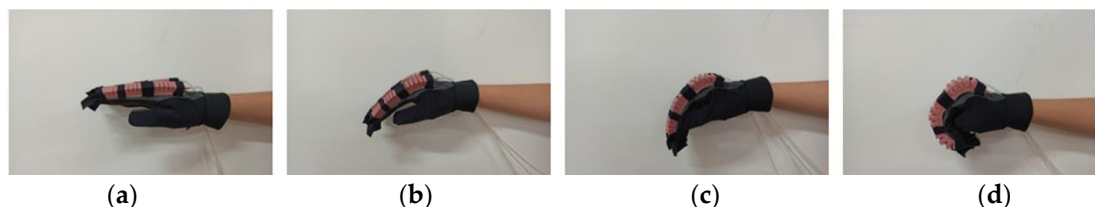
Figure 13. The four wearing states of sExoG. (a) Extension, (b) Rest, (c) Spherical grip, (d) Fist.
